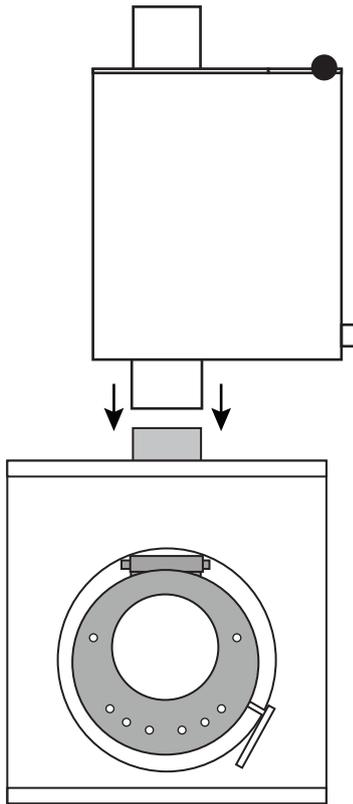
1. Lift the water heater on to the top of the stove. The hinged lid with a handle should be facing upwards and the pipe that goes through the tank must be fitted tightly over the stove's flue pipe.
