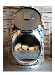
**NOTE** that the stove door may change color after a while in use and the paint may wear off. The door can be repainted with heatproof paint that can withstand temperatures up to 600 degree Celsius. Before painting the door, the surface must be polished and wiped clean of all traces of oily substances.
