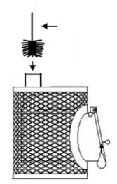
Remove the upper mesh frame and detach the pipe. Sweep the fire pipe following the directions given above with the Original IKI and Maxi IKI. Dismantling, sweeping and assembling the stove takes 1–2 hours all in all.
