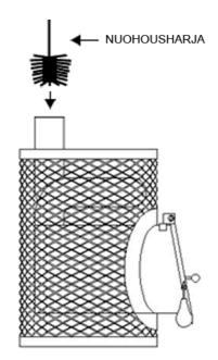
2. Spray or pour water into the pipe and use a sweeping brush to clean the inside of the smoke pipe. Note that the spiral smoke pipe requires a brush that bends.
