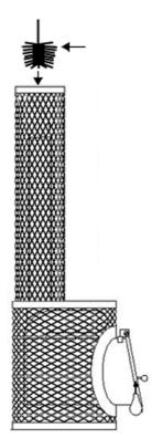
Remove the stones from the upper mesh frame until you reach the connection to the smoke pipe. Detach the pipes.
