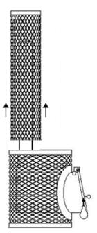
If the sweeping brush is short, continue removing the stones from the upper part of the mesh frame. When you no longer reach the stones from above, slide the frame upwards and start removing the stones from underneath it.
