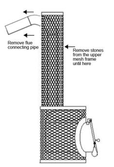
Remove flue connecting pipe
