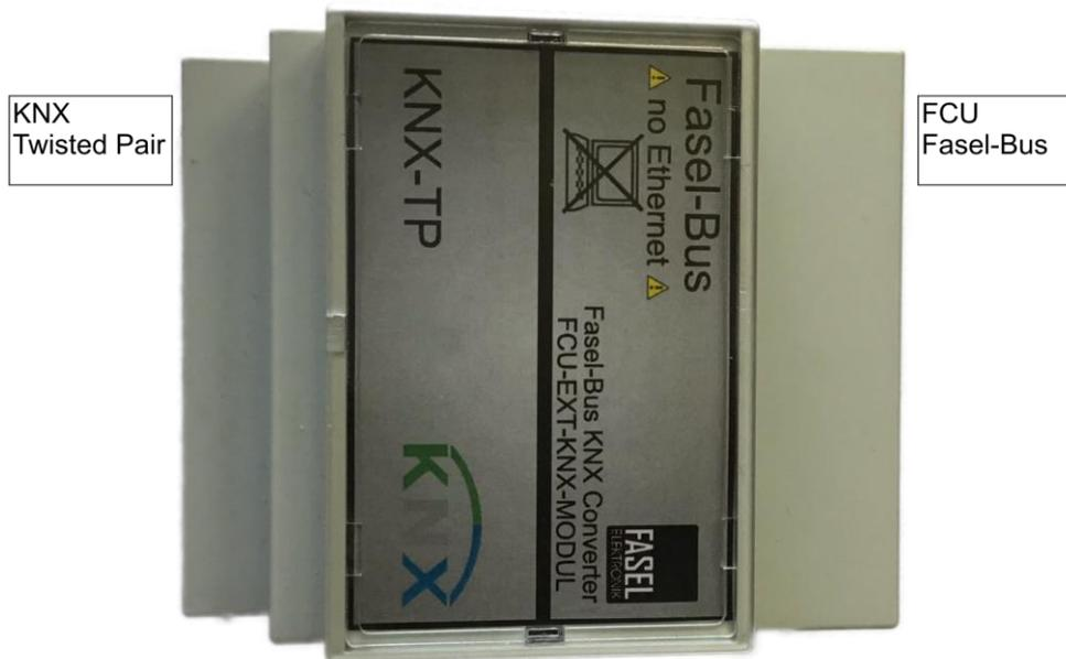
Connections of the KNX Module.
